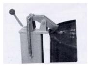
Then push the bulbous knob that is connected to clamp (Part No.1) so as for the clamp to bite the drum firmly and for the bulbous knob to lock the clamp (Part No.1). Continue to pump up the lifting frame (Part No.2) by handle (Part No.4) and then the drum will be lifted.
